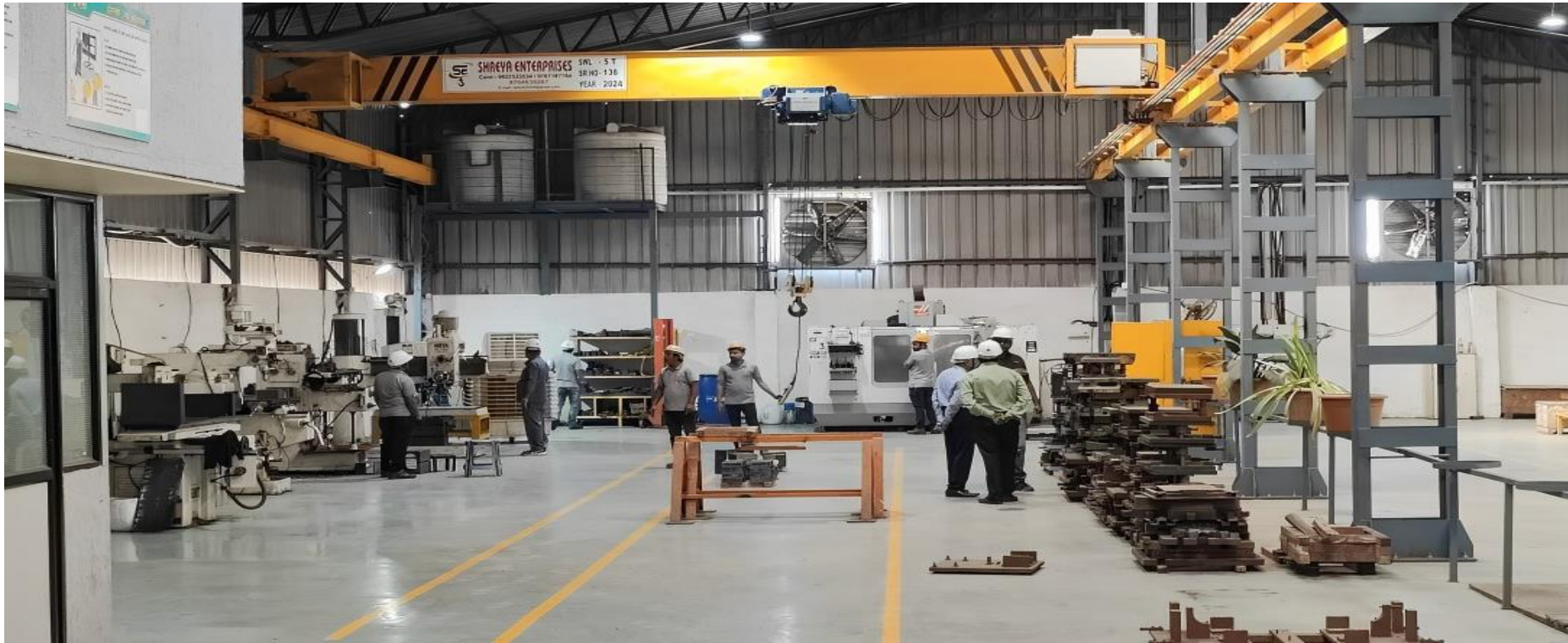
Commercial Tool Room Facility with 5 Ton Overhead Crane
